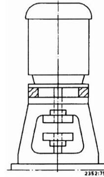
Fig. 16 – Decoupled drive
