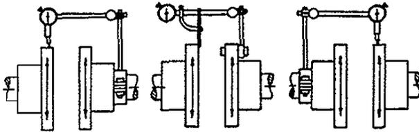
Fig. 12 - Aligning a spacer-type coupling with a dial micrometer
