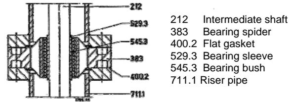
Fig. 05 Intermediate shaft bearing
