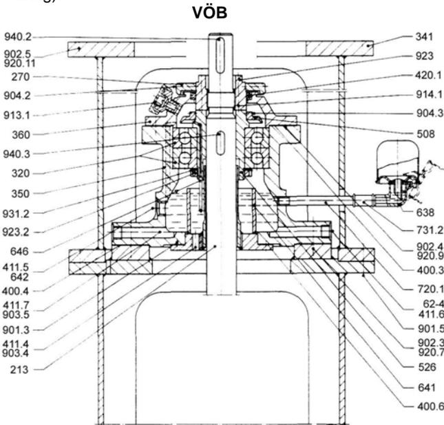
Fig. 08 Construction of support bearing VÖB
