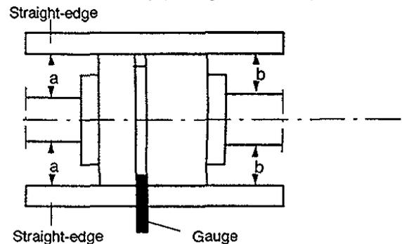
Fig. 10 - Aligning the coupling with the help of a gauge and a straight-edge
