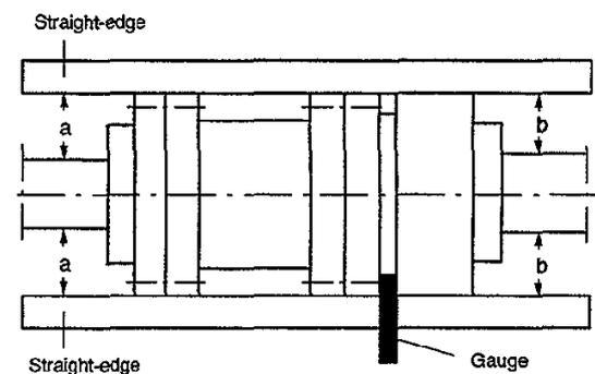
Fig. 11 - Aligning a spacer-type coupling
